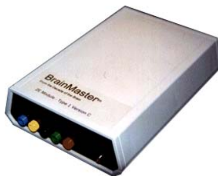
Figure 6-2: Picture of the Brainmaster EEG Module used in the development of the Affective Choice system, (Thomas F. Collura [12])
