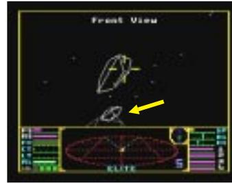
Figure 13: The visibility determination algorithm employed by *Elite* resolved local visibility only via back-face culling. Note the incorrect visibility indicated by the arrow.
